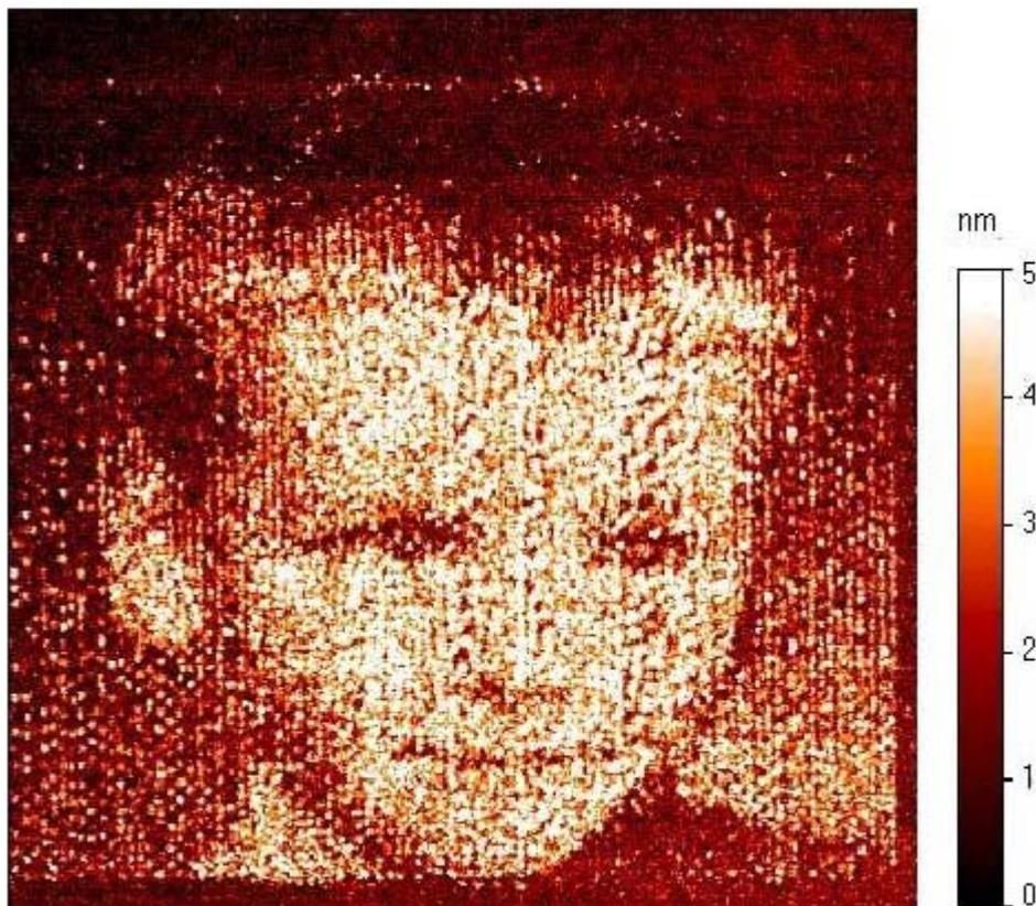
Fig.: STM image of graphite-like nanodots within a diamond-like carbon layer (image size  $1.2 \mu\text{m} \times 1.2 \mu\text{m}$ ).
