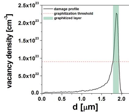
Fig. 1. Damage density profile (black continuous line) for a 1.1 MeV  $\text{He}^+$  implantation at a fluence of  $1 \cdot 10^{17} \text{ cm}^{-2}$ . The graphitization threshold is reported in the dashed line. The graphitized layer formed upon thermal annealing is highlighted in the box.
