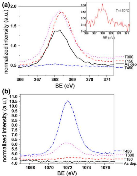
**Fig. 6** Silver ( $\text{Ag } 3d_{5/2}$ ) (a) and sodium ( $\text{Na } 1s$ ) (b) XPS peaks in silver nanocluster/silica composite coatings on soda-lime glasses as-deposited and after thermal treatments. The *inset* shows the spectra after the annealing at 450 °C. The *curves* have been normalized to the intensity of the Si 2p peak
