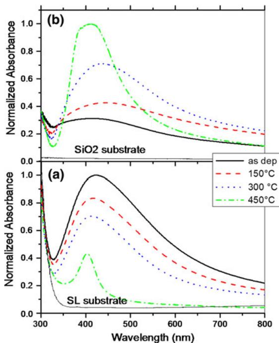
**Fig. 3** UV-Vis absorption spectra of silver nanocluster/silica composite coatings on soda-lime (a) and silica (b) substrates, evidencing the silver nanoclusters Localized- Surface Plasmon Resonance absorption peaks, as-deposited and after thermal treatments. The curves are normalized to the maximum of the as-deposited sample for the coatings on soda-lime and to the maximum of the sample heated at 450 °C on SiO<sub>2</sub>
