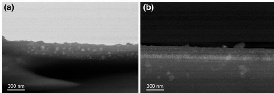
**Fig. 2** FESEM on silver nanocluster/silica composite coating cross section on soda-lime glasses as-deposited (a) and after thermal treatment at 450 °C (b)
