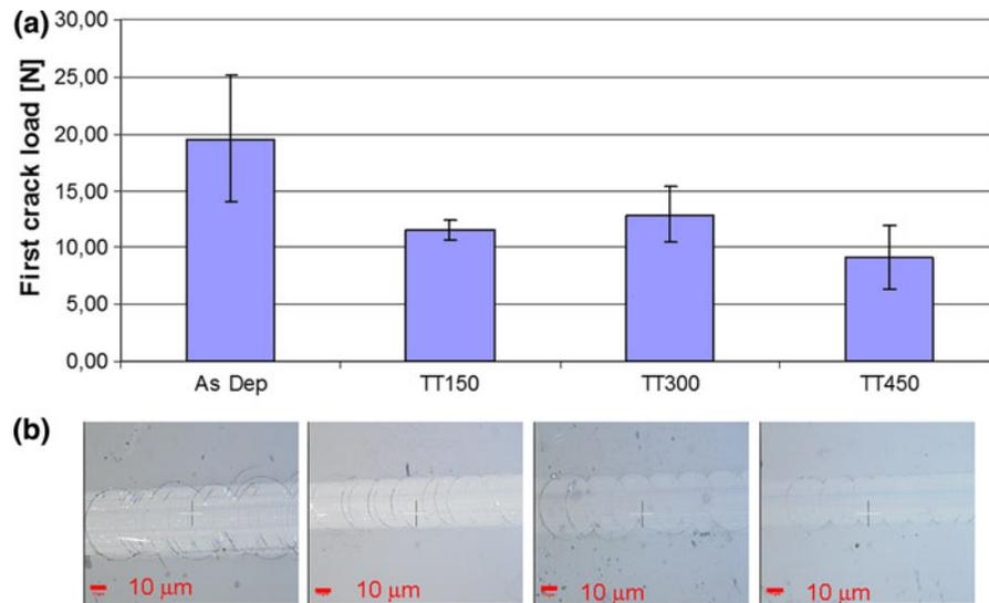
**Fig. 9** Scratch tests on silver nanocluster/silica composite coatings on soda-lime glasses before and after thermal treatment: **a** comparison of first crack load and **b** morphology of the first crack
