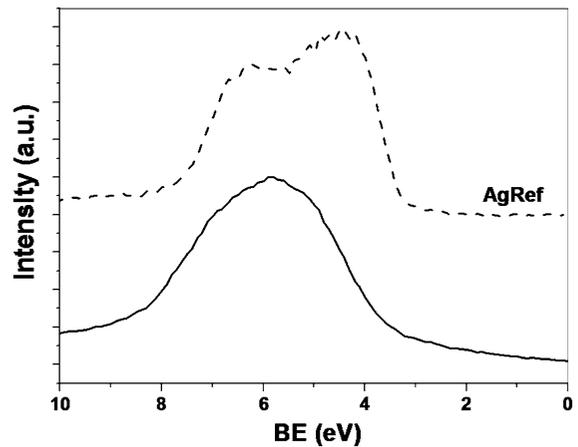
**Fig. 14** XPS valence band of the silver nanocluster/silica thin film as-deposited on a silicon substrate measured using a Scienta ESCA 200 analyzer (Gammadata, Sweden) equipped with a monochromatized  $\text{Al K}_{\alpha}$  X-ray source (pass energy 300 eV, step size 0.1 eV). The upper spectrum, shown for comparison purposes, is a reference silver metallic thin film ( $\text{AgRef}$ )
