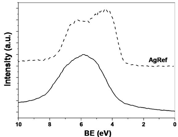
**Fig. 14** XPS valence band of the silver nanocluster/silica thin film as-deposited on a silicon substrate measured using a Scienta ESCA 200 analyzer (Gammadata, Sweden) equipped with a monochromatized  $\text{Al K}_{\alpha}$  X-ray source (pass energy 300 eV, step size 0.1 eV). The upper spectrum, shown for comparison purposes, is a reference silver metallic thin film (AgRef)
