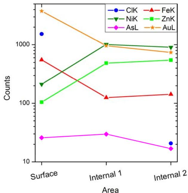
Fig. 3. Distribution of minor elements between surface and bulk areas (the analysed areas are shown in Fig. 2).
