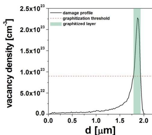
**Fig. 1.** Damage density profile (black continuous line) for a 1.1 MeV He<sup>+</sup> implantation at a fluence of  $1 \cdot 10^{17} \text{ cm}^{-2}$ . The graphitization threshold is reported in the red dashed line. The graphitized layer formed upon thermal annealing is highlighted in the green box.
