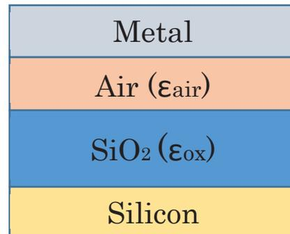
Fig.9: Dielectric stack between metal and silicon.
