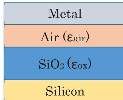
Fig.9: Dielectric stack between metal and silicon.
