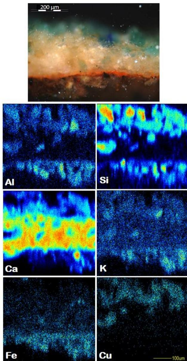
Fig. 1. Optical microscope image of the sample C1 in cross section (top) and  $\mu$ -PIXE acquisitions on a  $500 \times 500 \mu\text{m}^2$  scanned area. All reported PIXE maps are equally scaled in dimension and highlight the layering sequence. Color scale is from black (minimum value) to red (maximum value).
