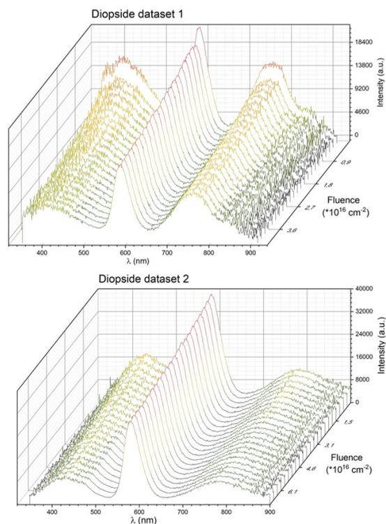
Fig. 2. Evolution of IBIL spectrum of the diopside crystal as a function of the fluence for the two datasets.
