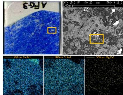
Fig. 1. (Up) Petrographic section of the rock sample (left) and SEM-BSE (right) image acquired in the area of the target diopside crystal and highlighted by the yellow box. (Down) PIXE maps of Ca, Si and Mg acquired on the crystal.
