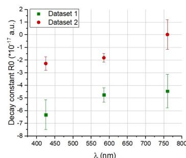
Fig. 4. Decay constant R0 parameters obtained from the exponential fit of the data shown in Fig.3 for the two datasets.
