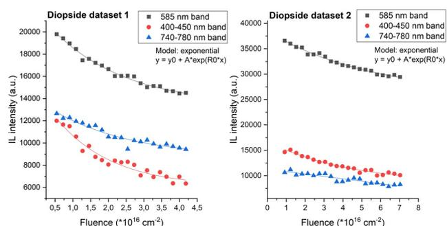
Fig. 3. Evolution of the peak intensity of the main bands in diopside spectra as a function of the fluence for the two datasets. The expression of the exponential curve used for the fitting procedure is reported.
