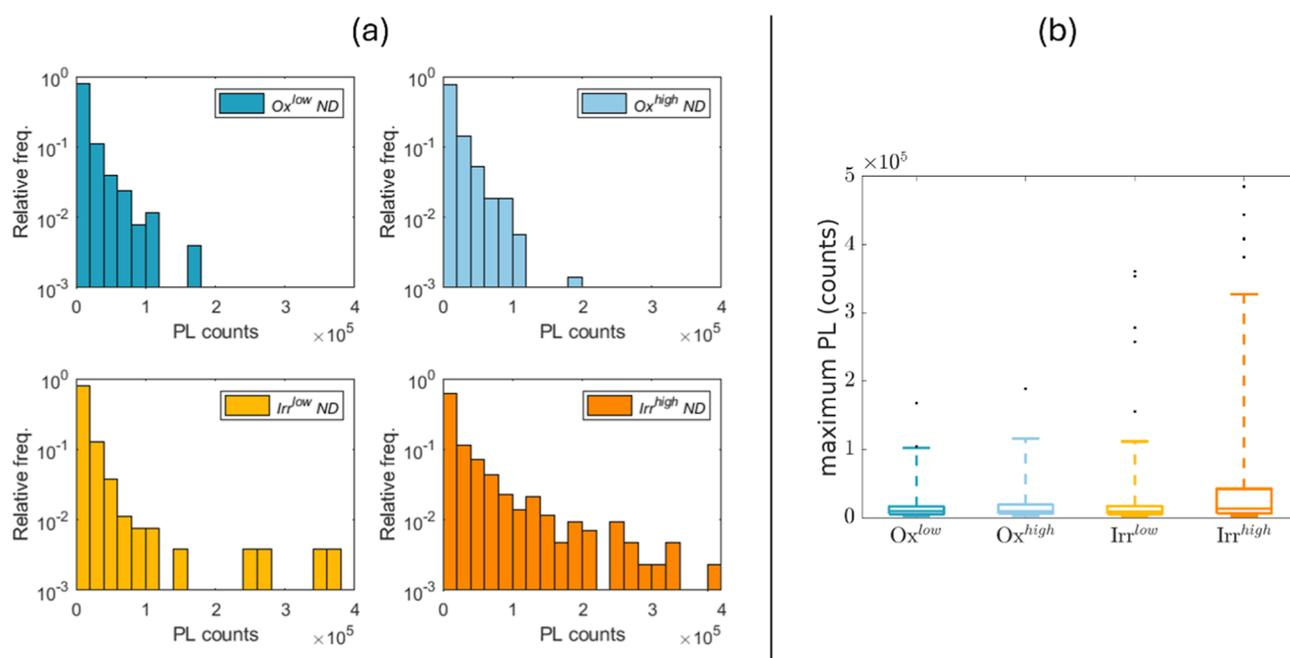
**Figure 7.** (a) Normalized histograms reporting the maximum PL distribution in the different ND samples. (b) Box and whisker plot of the PL counts in the different NDs samples. Data are obtained from isolated NDs (>300 in each case), identified on PL maps (as the one reported in Figure 6) acquired at our home-built scanning confocal setup.
