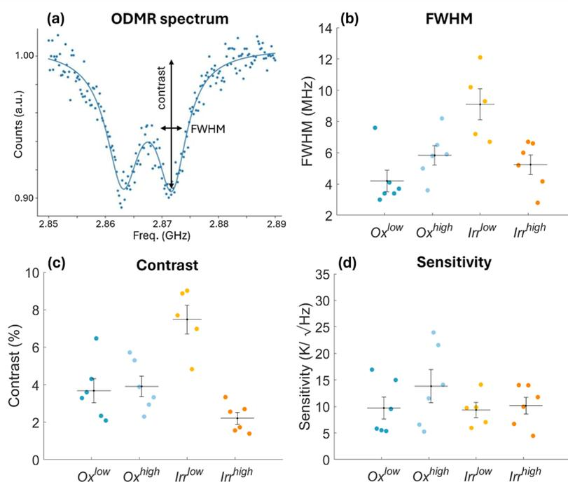
**Figure 8.** (a) Example of ODMR spectrum from an  $\text{Irr}^{\text{high}}$  ND, normalized and fitted with a double Lorentzian curve. (b) fwhm, (c) contrast, and (d) shot-noise limited sensitivity (according to eq 1) for several NDs in the different samples.
