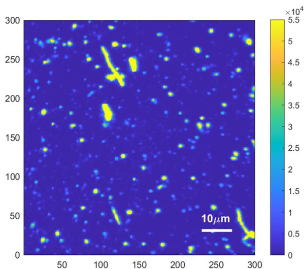
**Figure 6.** PL map acquired at our home-built scanning confocal setup for the  $Ox^{low}ND$  sample. The area measures  $(80 \times 80) \mu m^2$  scanned with a resolution of  $(300 \times 300)$  pixels.
