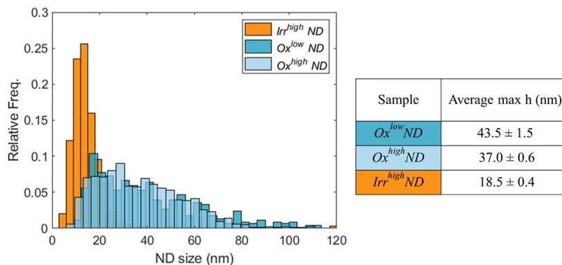
**Figure 5.** Normalized histograms reporting the diameter distribution for different ND samples (*Irr*<sup>high</sup>ND, *Ox*<sup>high</sup>ND, and *Ox*<sup>low</sup>ND), according to AFM analysis. The table reports the average size and associated standard deviation in the different cases.
