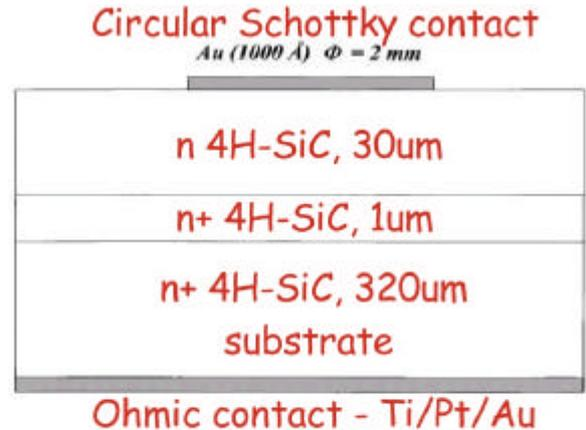
Fig.1 SiC Schottky diode geometry.
