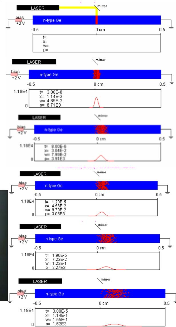
If an amount of net charge is injected suddenly in a semiconductor, the free charge carriers of opposite sign try to balance the injected charge and establish charge neutrality.
