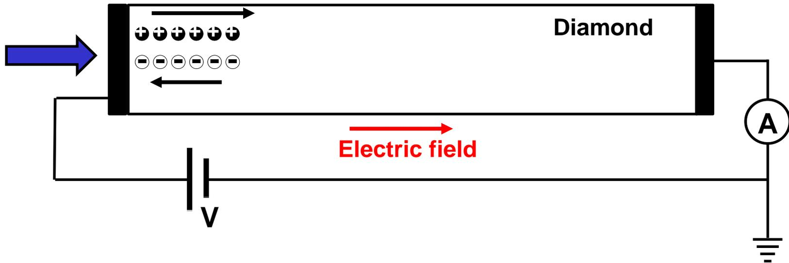
Charge carriers (electrons-holes) generated by a ionizing particle move in an external electric field and **induce** charge on the electrodes
