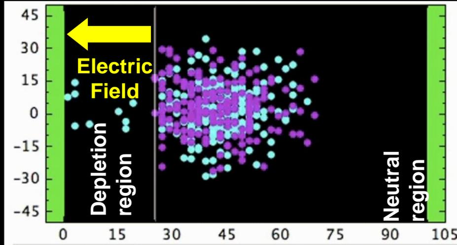
Only holes injected in the depletion region by diffusion induce a charge
