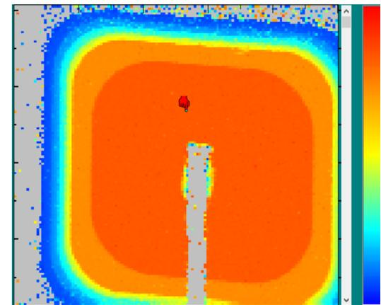
Modulation of the carrier generation profiles by different widths of the depletion region induced by changing the applied bias voltage
