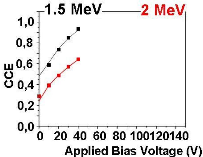
$$Q = Q_{\text{Depl}} + Q_{\text{Neutr}} \propto \left[ \int_0^w \left( \frac{dE}{dx} \right) \cdot dx \right] + \left[ \int_w^d \left( \frac{dE}{dx} \right) \cdot \exp \left[ -\frac{x - W}{L_p} \right] \cdot dx \right]$$
