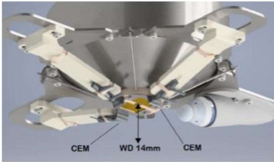
**Figure 1.** Ionoptika Ltd. detector array on the SIMPLE tool. Labelled are the CEMs that collect the SE signal. These are positioned on the nose cone of the ion gun at a 10 mm distance from the implant site. The working distance of the tool is 14 mm.
