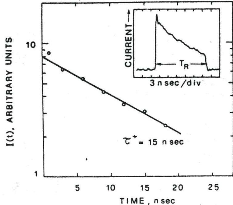
Drift velocity;  $v = \mu E = d/T_R$
