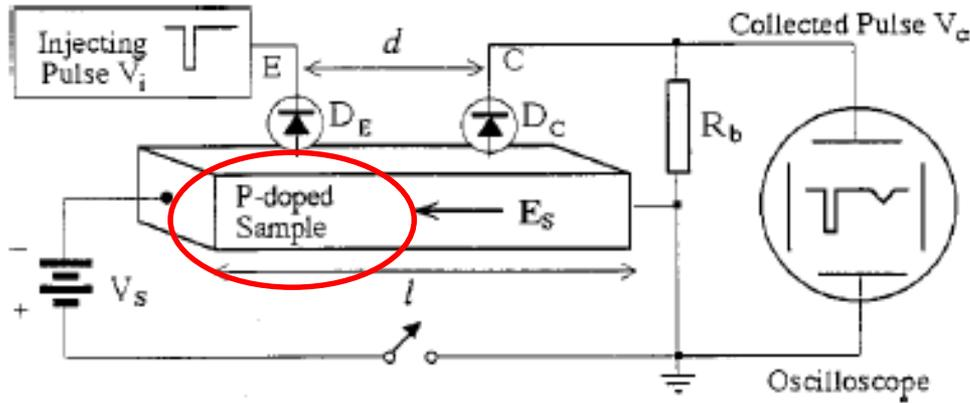
Fig. 1. Block diagram of the Haynes Shockley experiment:  $D_E$  and  $D_C$  are the emitter and collector point probes.
