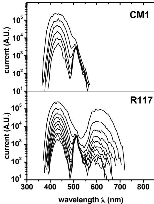
Fig. 1 - IBIL spectra of CVD diamond samples CM1 and R117 as recorded at increasing times. IBIL intensity continuously decreases. Each spectrum corresponds to about  $10^{15}$  p/cm<sup>2</sup> of proton dose over a surface area of  $0.5 \times 0.5$  mm<sup>2</sup>. Sample R117 is characterized by a poorer charge carrier collection efficiency with respect to the sample CM1.
