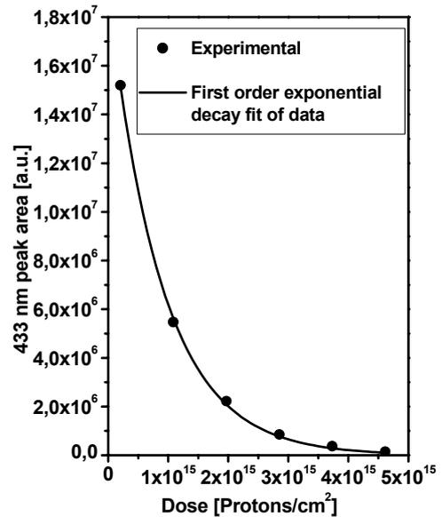
Fig. 2 - Decay of the A band intensity as a function of proton dose. The intensity has been calculated as the total area under the peak at 430 nm.
