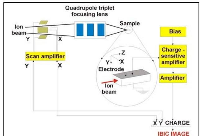
FIG. 1: lateral IBIC Set up
