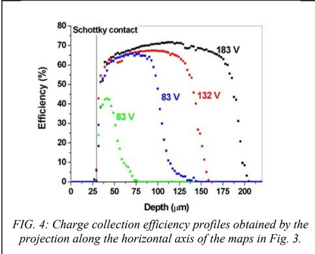
FIG. 4: Charge collection efficiency profiles obtained by the projection along the horizontal axis of the maps in Fig. 3.
