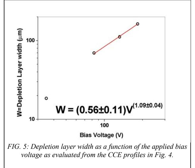
FIG. 5: Depletion layer width as a function of the applied bias voltage as evaluated from the CCE profiles in Fig. 4.
