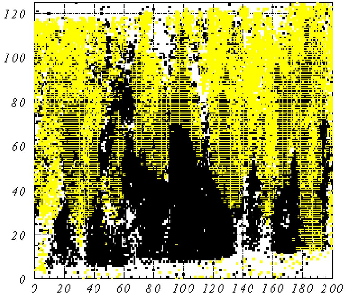
Superimposed IBIC ( yellow ) and IBIL ( black ) maps obtained irradiating the cross section of a CVD diamond film (400  $\mu\text{m}$  x 800  $\mu\text{m}$ ). Growth side is at the top, substrate side is at the bottom.
