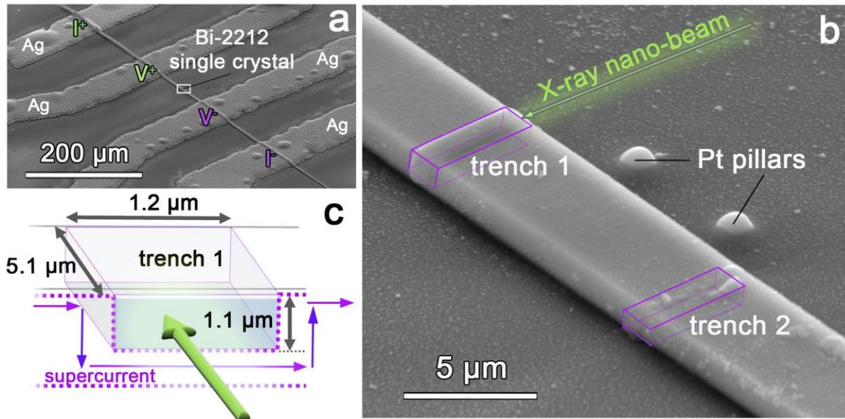
Experimental setup for X-rays nanopatterning experiments. a) Bi-2212 single crystal on a sapphire substrate, with 4 Ag electrodes for electrical measurements, b) example of irradiated regions acting like « trenches » for the current path, and c) sketch of the modifications induced by X-rays irradiation in the current path around a « trench ». Pt pillars are just markers for alignment purposes.
