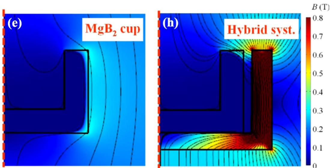
Magnetic field distribution in the case of applied magnetic field  $\mu_0 H = 0.2\text{T}$  in the case of purely superconducting (e) and of hybrid superconducting/ferromagnetic (f) cylindrical coaxial cups.
