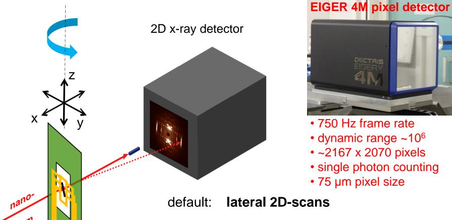
750 Hz frame rate dynamic range ~10<sup>6</sup> • ~2167 x 2070 pixels single photon counting 75 µm pixel size
