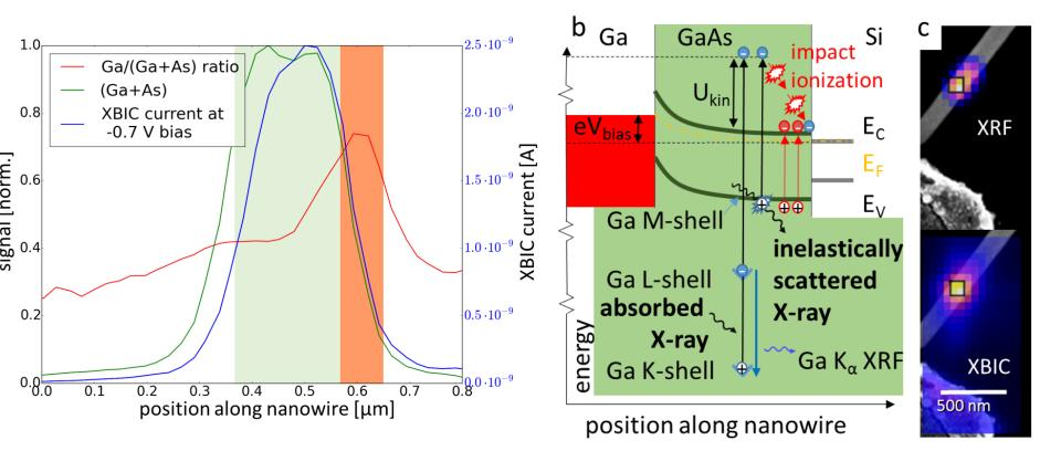
With a bias or intrinsic field X-ray Beam induces a current (XBIC)
