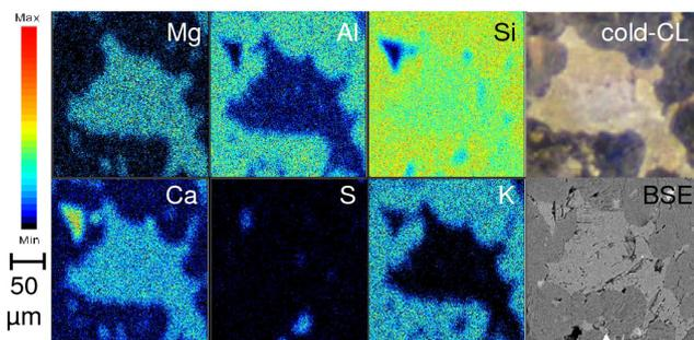
Fig. 2.  $\mu$ -PIXE elemental maps (the inclusion in the map is composed by calcium, magnesium and silicon that are the main elements of diopside), BS Electron Microscopy and cold-cathodoluminescence images.
