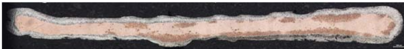
Fig. 1. Sections of an ancient Roman republican coin Victoriatus at the optical microscope (5X). Reference bar: 500 \mu\text{m} .
