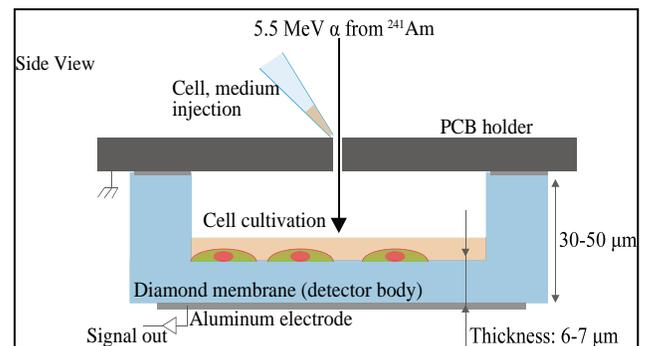
Fig.1. Schematic illustration of diamond membrane with cell cultivation condition.
