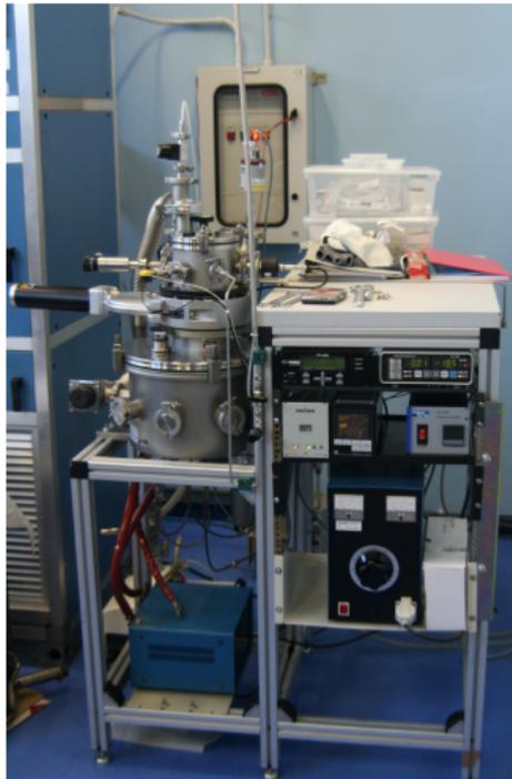
Figure: Deposition of Ni-films system at I.N.Ri.M.
