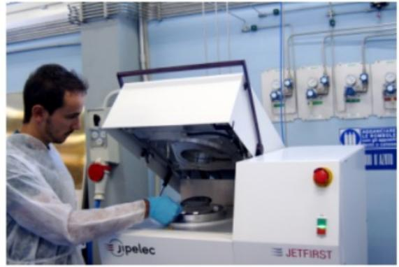
**Figure:** RT-CVD system at I.N.Ri.M. - highest temperature reached: 1300 °C,
